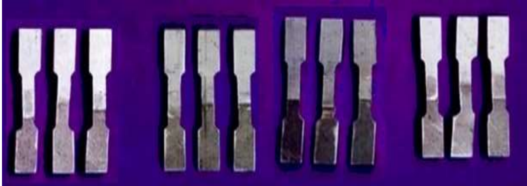
Figure. 2. Tensile strength specimens of FS welded AA 7075 with AA 6063
