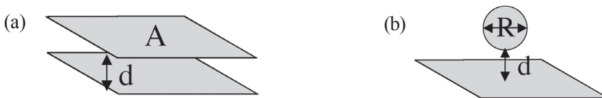
Figure 3. Plate-plate and sphere-plate Casimir force measurements.
