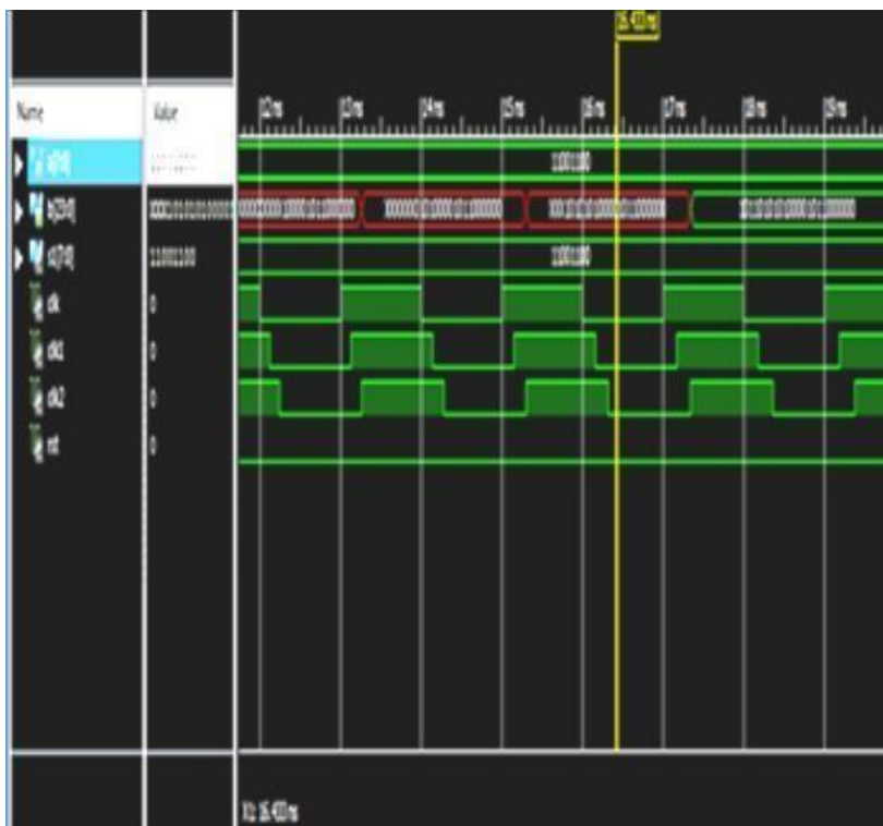
Fig. 3: Encoder output wave forms
