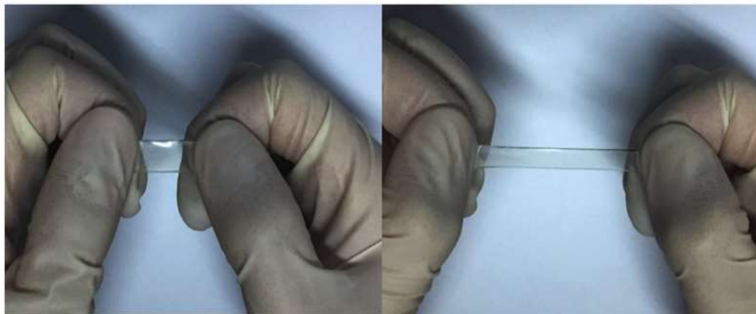
Figure 4 snapshot of stretching of poly(urethane-acrylate) elastomer (MA:BA mass percentage ratio of 100:0 [23]
