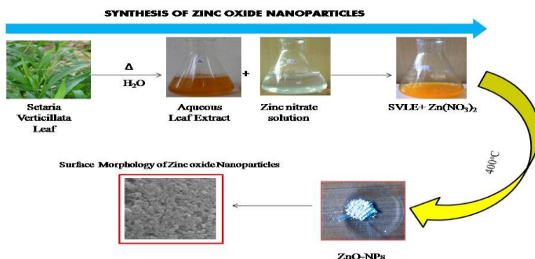
Figure 1. Schematic synthetic route of Zinc oxide nanoparticles.
