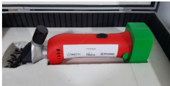
Fig. 6: Clipper with 12 volt adaptation
