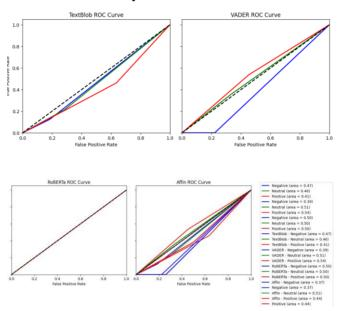
This image shows the receiver operating characteristic (ROC) curves for four different sentiment analysis models: TextBlob, VADER, RoBERTa, and Affin. Each plot evaluates the differences between the false positive and true positive rates for various classes: negative, neutral, and positive sentiments.
