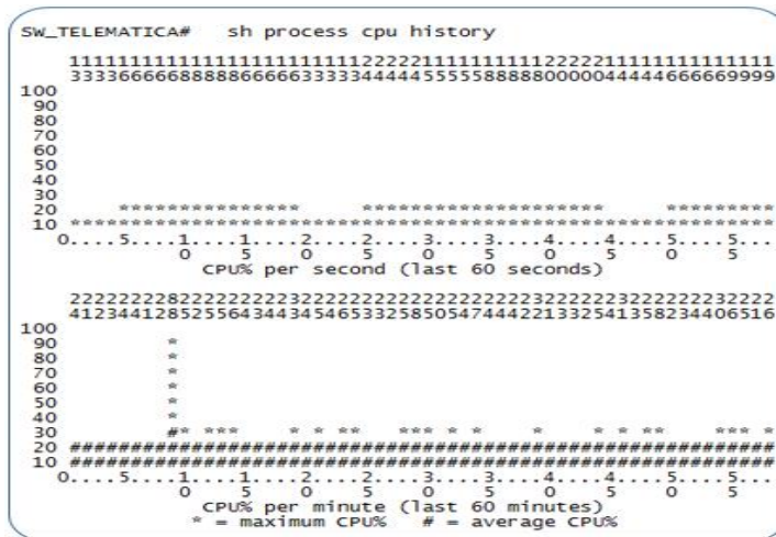
Figure 8. Switch Core CPU utilisation in the absence of MAC flapping
