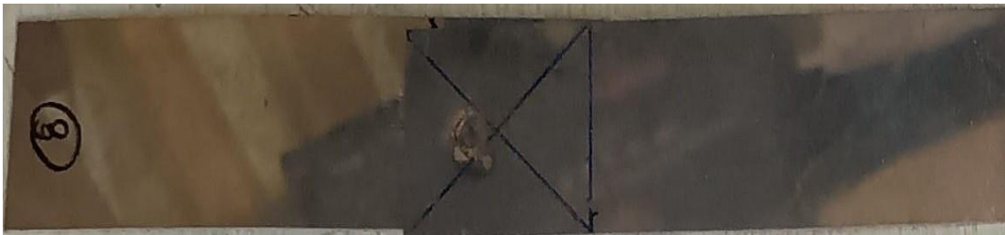
Figure 1(b): Photograph of tensile shear strength specimen
