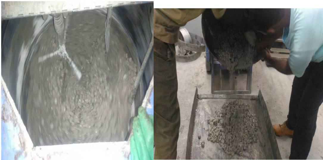
Figure 1: Mixing of concrete in pan mixer
