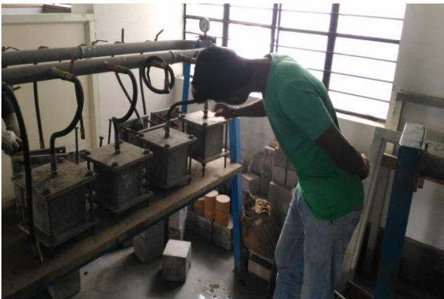
Fig 7: Permeability test apparatus and arrangement
