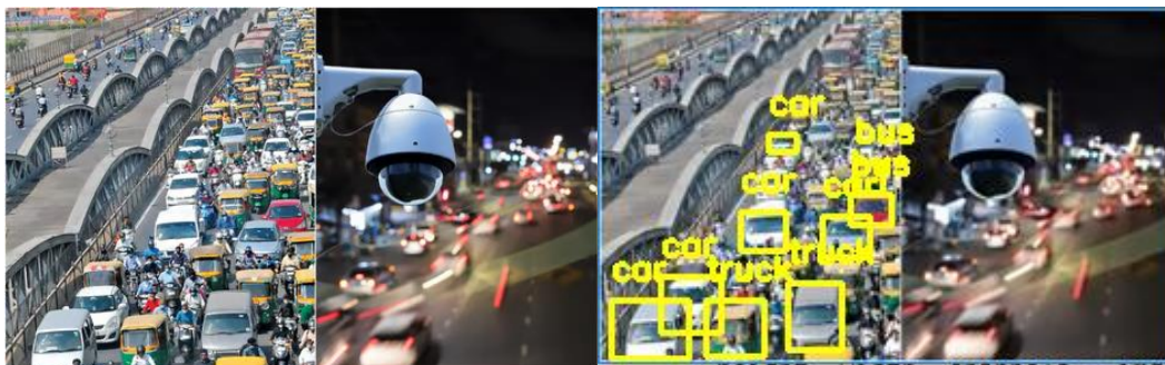
Fig:1 Detecting the objects using OpenCV library and YOLOv3
