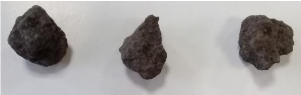
Figure 4. EAF black slag sample
