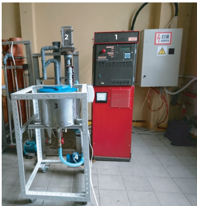
Figure 1. EED dispersion installation: 1, generator; 2, reactor; 3, sedimentation tank; 4, pump for liquid.
