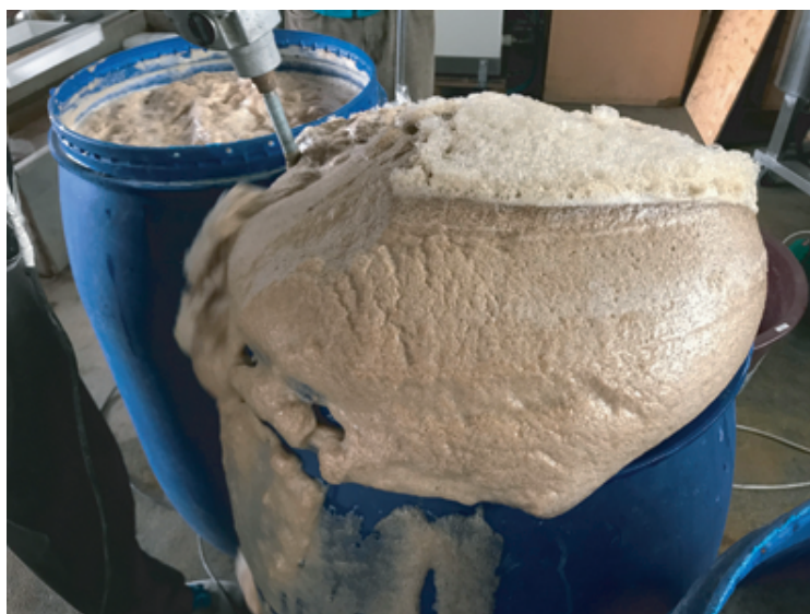
Figure 3. The foam formed as a result of destruction of heavy organic contaminants.
