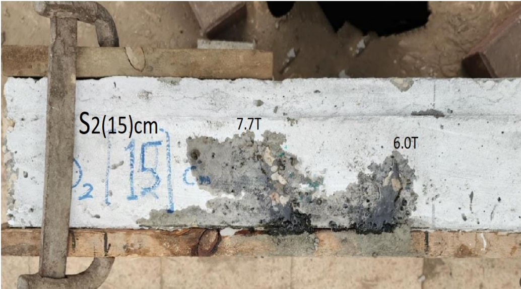
Figure 18: Repair of the concrete samples S2(10), S2(12) & S2(15) using Kema Epoxy 103
