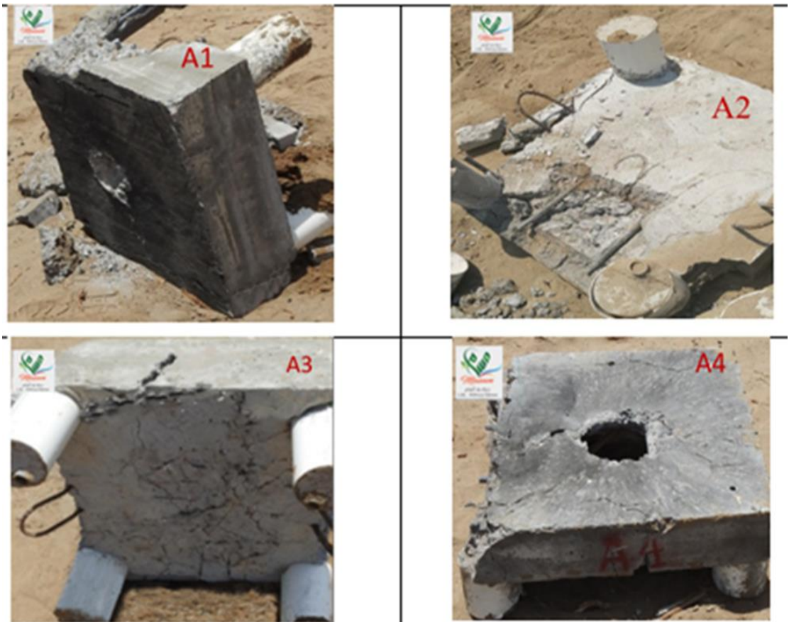
Figure 35: The damage of the concrete samples after being repaired and exposed to a second blast
