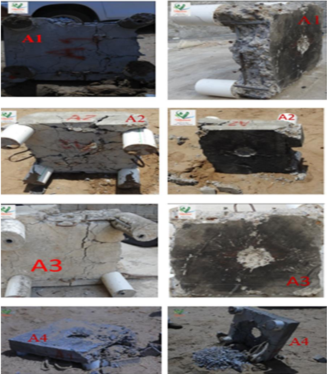
Figure 34: The damage of the concrete samples after being exposed to the first blast
