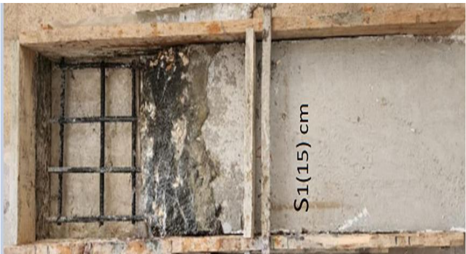
Figure 17: Repair of the control samples S1(10), S1(12) & S1(15) by using Citorex grout
