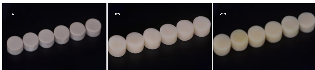
Figure 1: Sample preparation. A. PEEK samples (Group 1), B. PMMA samples (Group 2), C. Indirect composite sample (Group 3)
