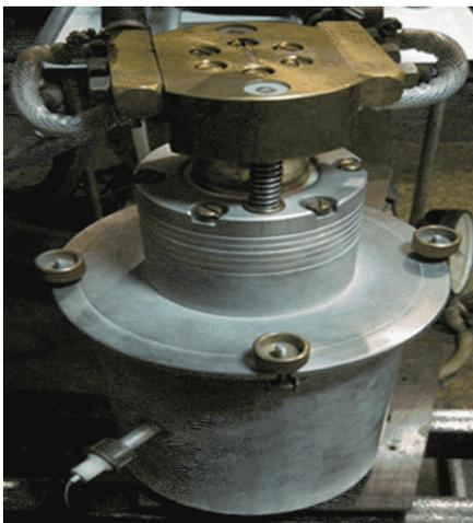
Figure 1. Vacuum chamber of the hot-pressing apparatus (electrical consolidation).<sup>7</sup>
