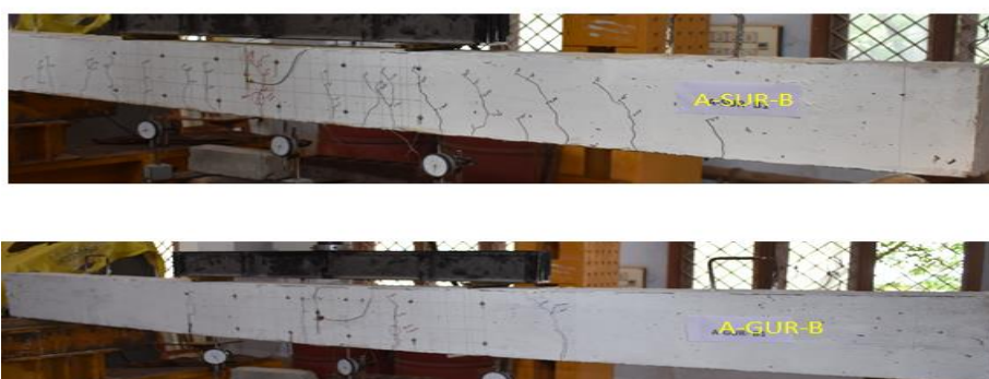
Figure: 6 Crack pattern of Alccofine replaced concrete
