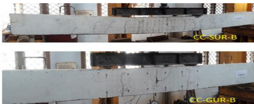
Figure: 5 Crack pattern of Conventional concrete
