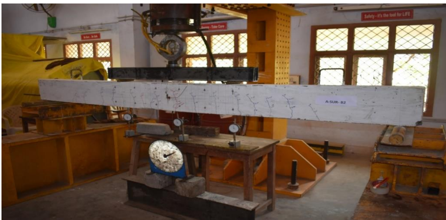
Figure:3 Experimental setup of testing the beam
