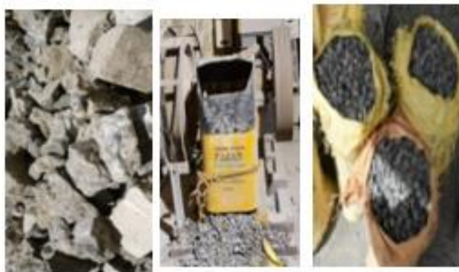
Figure 1. Preparation of recycled aggregate for concrete waste using jaw crusher.
