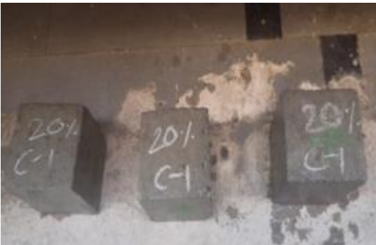
Figure 3. Concrete with 20% glass waste powder
