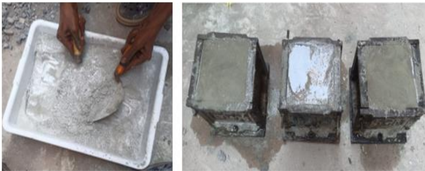
Figure 1. mixing and casting of specimens
