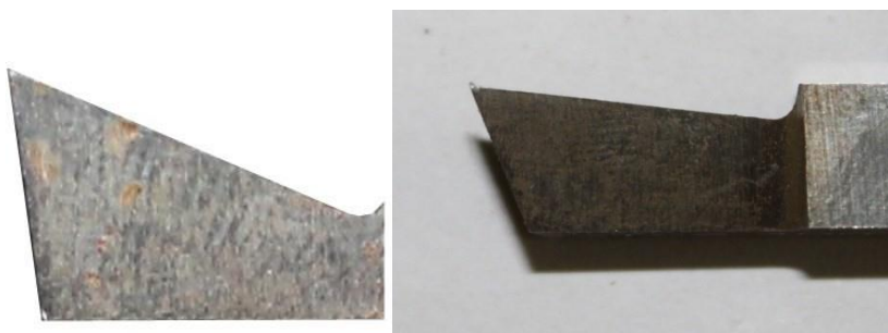
Figure 35: Tool-32 geometry before and after experiment
