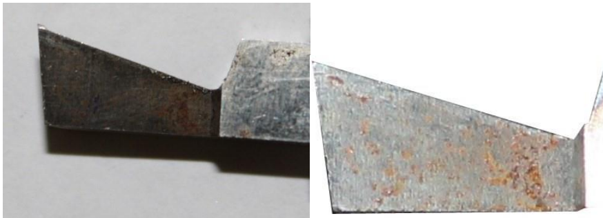
Figure 21: Tool-18 geometry before and after experiment
