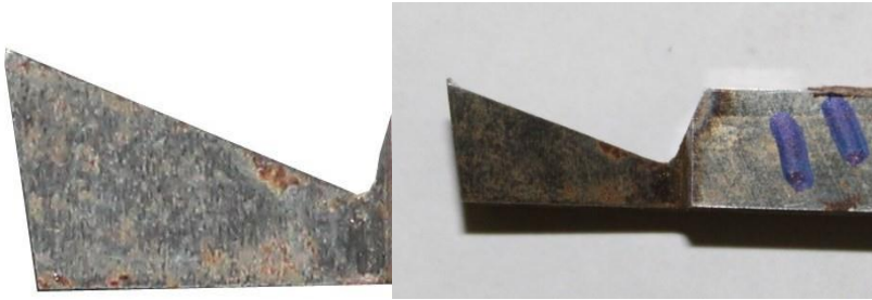
Figure 30: Tool-27 geometry before and after experiment
