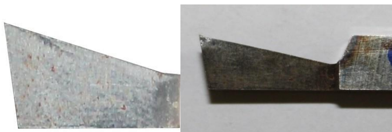
Figure 27: Tool-24 geometry before and after experiment
