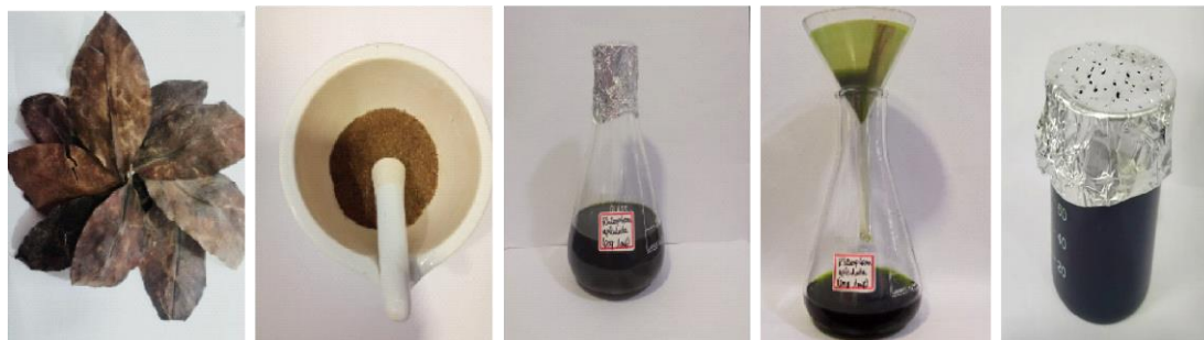
Figure 1: Extraction of marine bioactive compounds from Mangrove Rhizophora apiculata : a) Rhizophora apiculata leaf b) Powdered sample, c) Extraction d) Filtration e) Crude Extract
