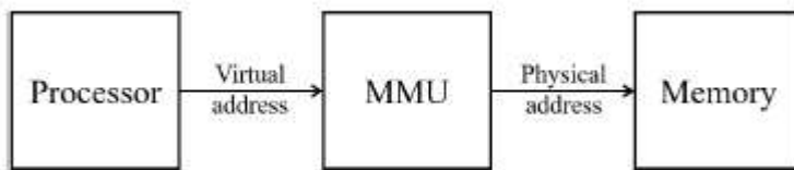
Figure 3.1 Conversion of virtual address into physical address in a hardware module
