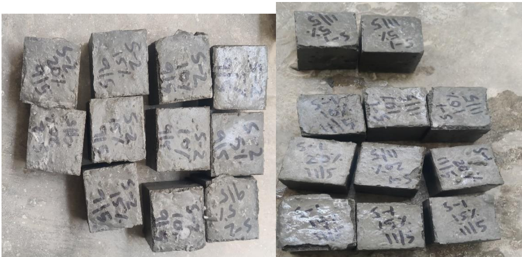
Figure 9: Cubes made with S1 and S2 Slag at different cement replacement percentage
