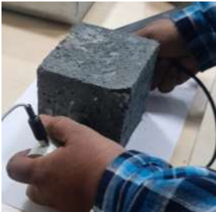
Figure F: Cross Probing Method of UPV Testing
