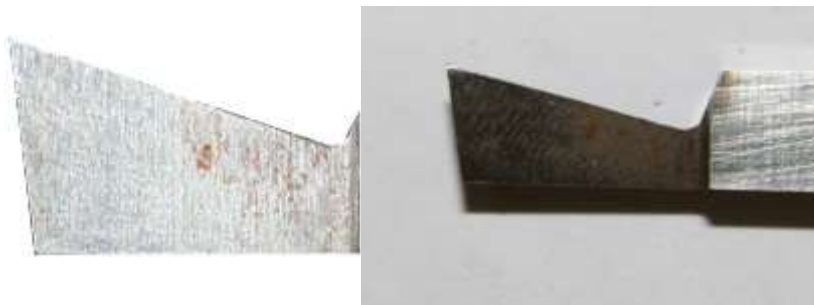
Figure 24: Tool-21 geometry before and after experiment
