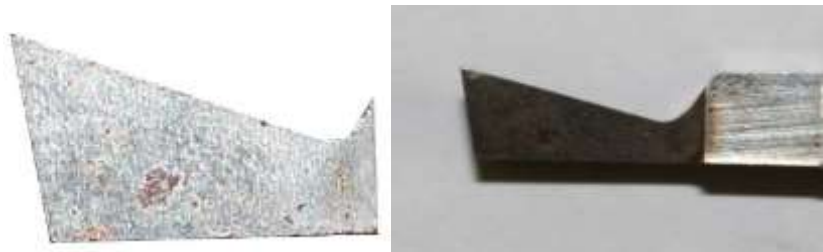
Figure 29: Tool-26 geometry before and after experiment
