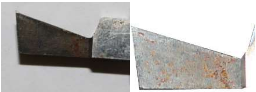
Figure 21: Tool-18 geometry before and after experiment
