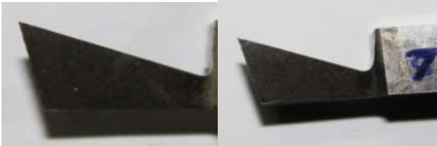
Figure 18: Tool-15 geometry before and after experiment
