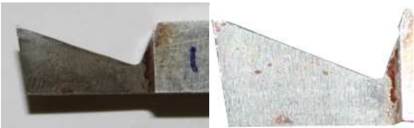
Figure 20: Tool-17 geometry before and after experiment
