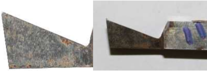
Figure 30: Tool-27 geometry before and after experiment
