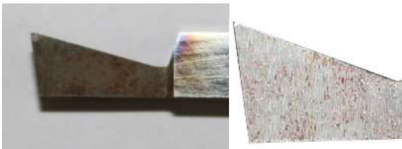
Figure 24: Tool-21 geometry before and after experiment
