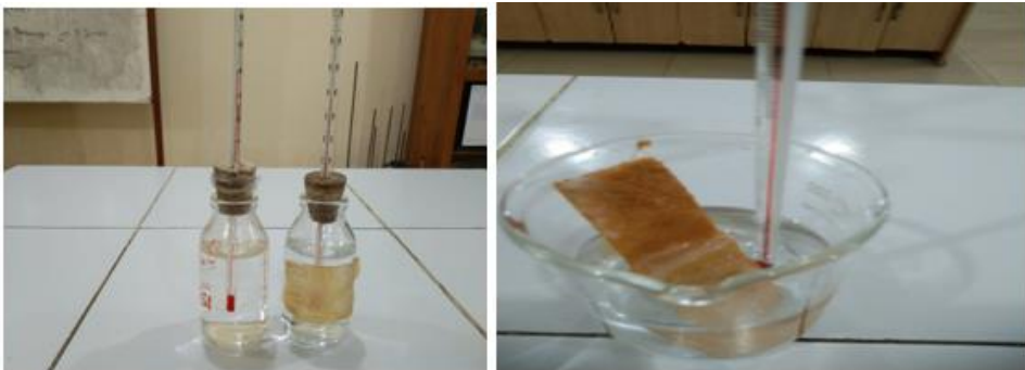
Figure 5 shows the heat adsorption capabilities of PCMs in open and closed containers resulting in the same trend change.
