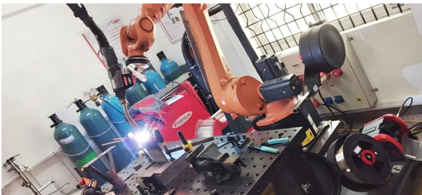
Figure 2.3 Automated-robotic CMT-WAAM set up
