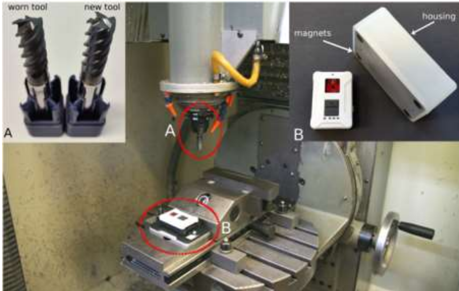
Fig. 1 CNC milling machine (a) New and worn tool (b) Magnetic mounting plate
