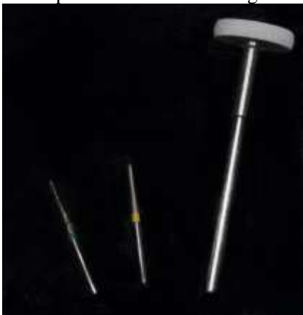
Figure 2: The polishing burs used in sequence for reglazing lithium disilicate blocks
