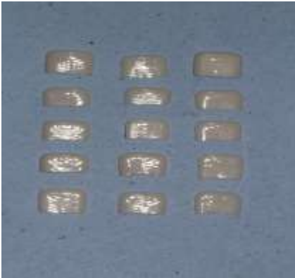
Figure 1: The samples prepared using used CEREC® blocks ( 0.5cm*1cm)
