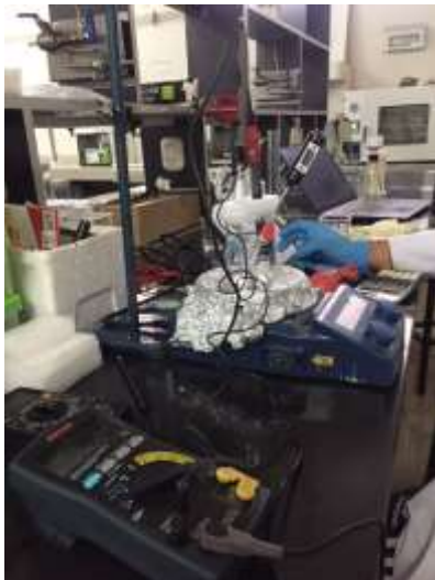
Fig. 3. Mounting the cyanide electrode
