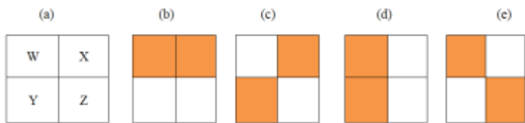
Figure 2: Four Texton types defined in MTH (a) 2 \times 2 grid (b) T_1 (c) T_2 (d) T_3 and (e) T_4
