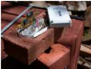
Fig. 21 Thermal sensor brick Source: [26].
