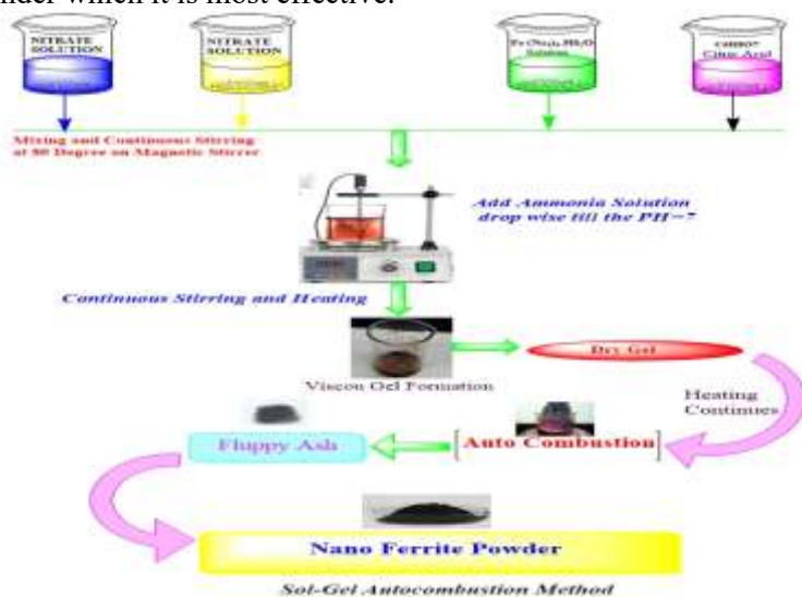
Fig. 1 Schematic representation of Sol-Gel Autocombustion Method
