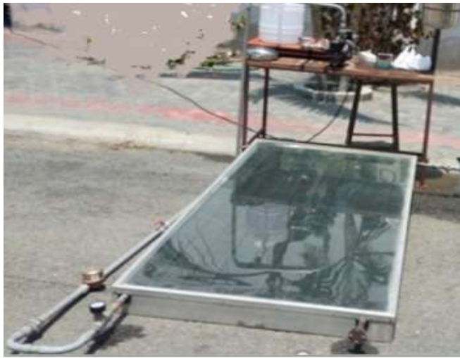
Figure 2. Experimental setup of solar flat plate collector.
