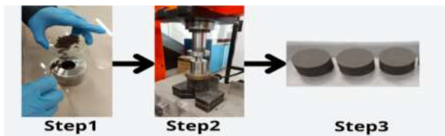
Figure 1 (a) Processing steps for making geopolymers
