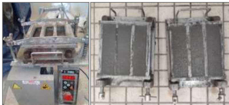
Figure 4. Impact table and specimen moulds (40x40x160) mm.
