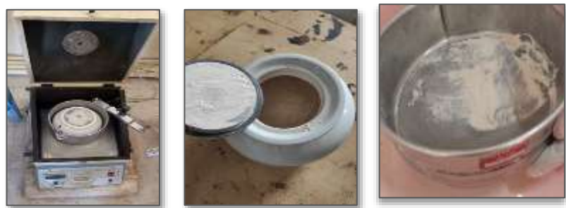
Figure 2. The crushing stages of dune sand.
