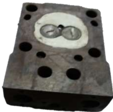
Figure 3: Photographic view of the ceramic coated cylinder head
