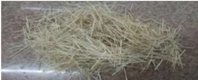
Figure 4: Bamboo fiber of diameter 1.156 mm Of aspect ratio ( l/d )=40 [10]
