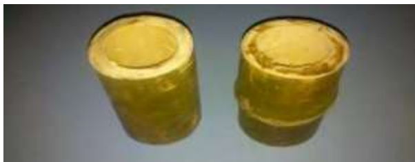
Figure 7: Bamboo samples in compressive strength test [84]
