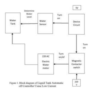
The device circuit activates the water sensor if the tank reaches its total capacity. On the other hand, the magnetic contactor will turn on until the water reaches its total capacity. The sensor signals the device circuit to switch off the electric motor once it reaches the tank's total capacity.
