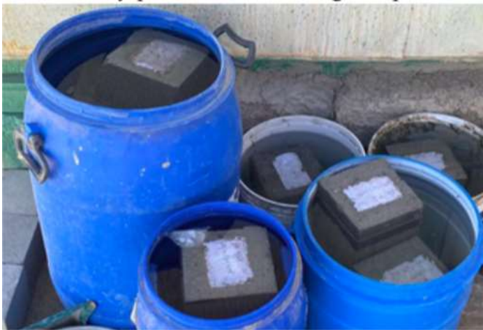
FIGURE 6 CURING OF CONCRETE SAMPLES FOR UP TO 7-DAY AND 28-DAY PERIODS
