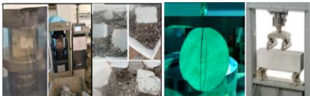
FIGURE 7 TESTING OF CONCRETE SPECIMENS FOR A) COMPRESSIVE TEST B) TENSILE TEST C) FLEXURE TEST
