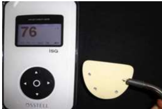
Figure 4: ISQ Value Measurement Using the Ostell Device
