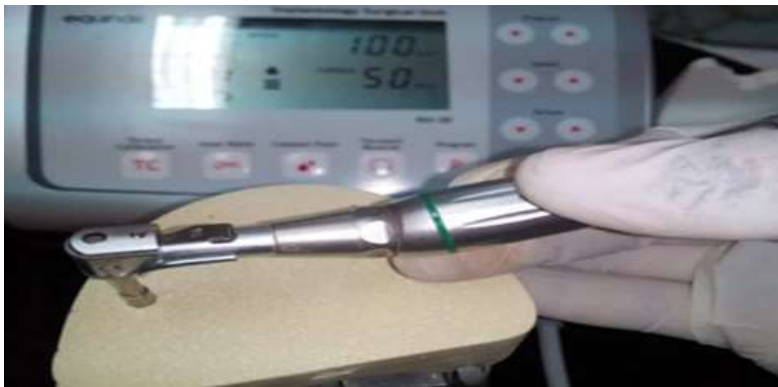
Figure 2: Insertion Torque Value measurement
