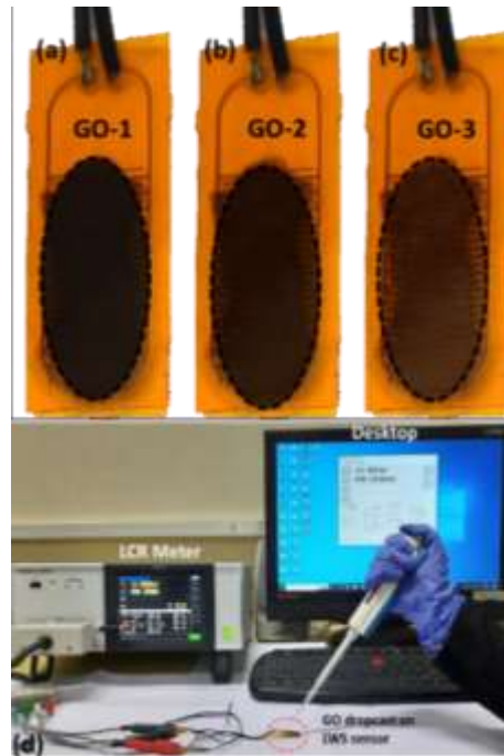
Fig. 1 Fabricated sensor on a flexible substrate with (a) GO-1, (b) GO-2, (c), GO-3, and (d) Experimental set-up
