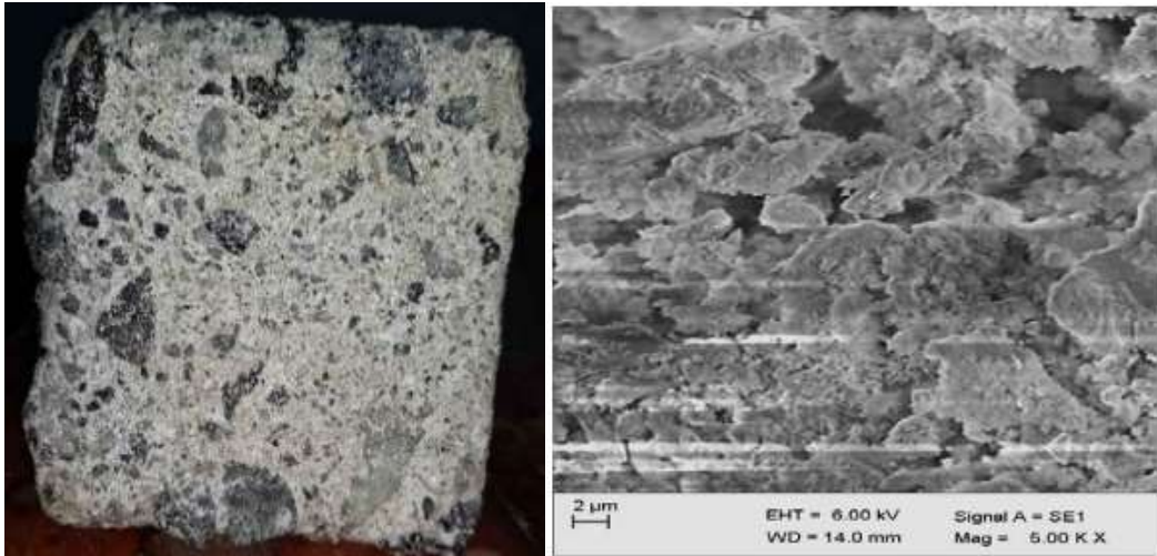
Figure: 5 Specimen dipped in 6M for 56 days
