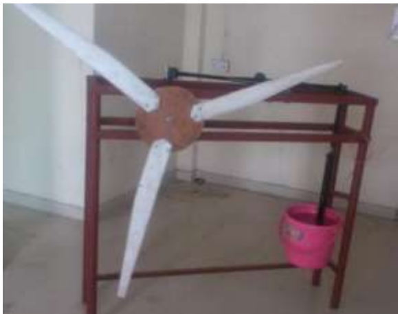
Fig.4 Prototype representation of wind operated single acting reciprocating pump
