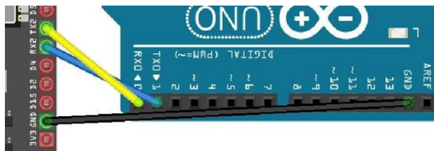
Fig. 4: Arduino and ESP Serial Communication.
