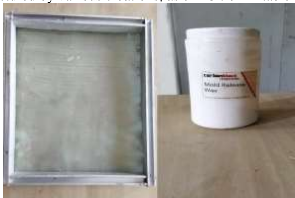
Figure.2: Aluminium mold and Mold release wax.
