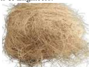
Figure 1: (a) Epoxy (LY-556) and Hardner (HY-951), (b) Treated Coir Fibre.
