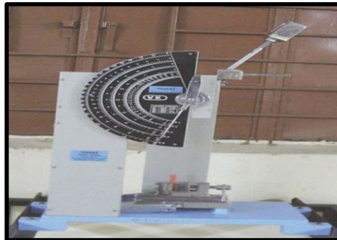
Fig.9 Impact Test on Izod Impact Test
