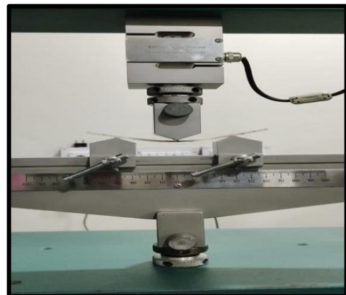
Fig.8Flexural Test on Universal Testing Machine
