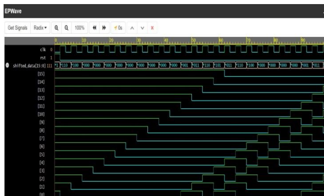
Fig 5.2. 16 Bit Seed Flip Ring Generator
