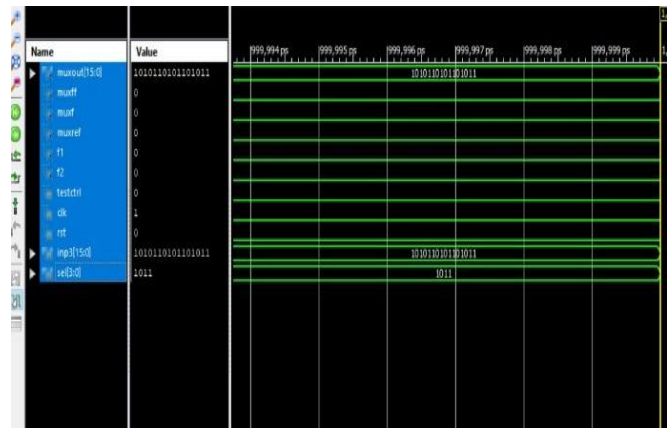
Fig 5.3. 16 Bit Test Pattern
