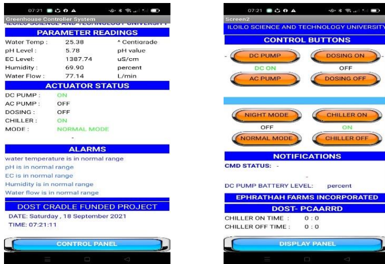
Figure 4. Screenshot of the developed android application software installed in the android mobile device showing the control panel (left) and the display panel (right).
