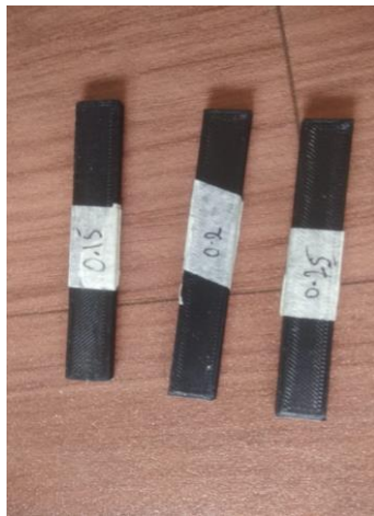
Fig: Specimens Are ABS(A) And PLA(B) Materials For Flexural Testing
