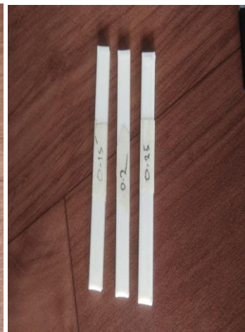
Fig: Specimens Are ABS(A) And PLA(B) Materials For Flexural Testing
