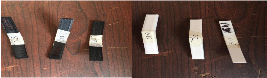
Fig: After Testing the Breaking Areas of Both ABS and PLA Materials
